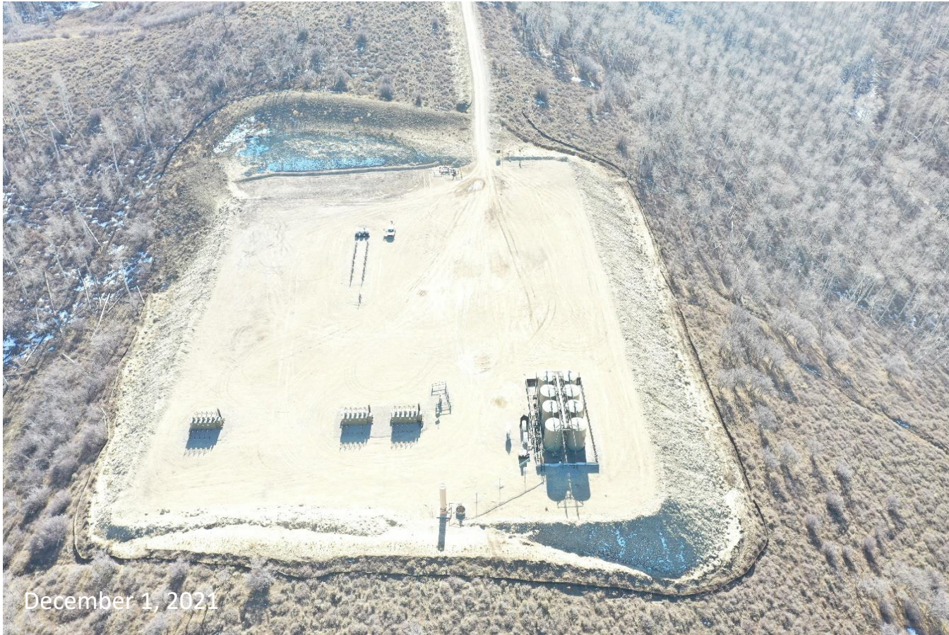
Photo 1: Photos 1-4 provide an aerial overview of the Location; Location disturbance ~6 acres. Photos show areas not needed for production have not been decompacted, recontoured/regraded and reclaimed; Location has not been reduced to 2 acres per the 2A Location Permit #401387622.
