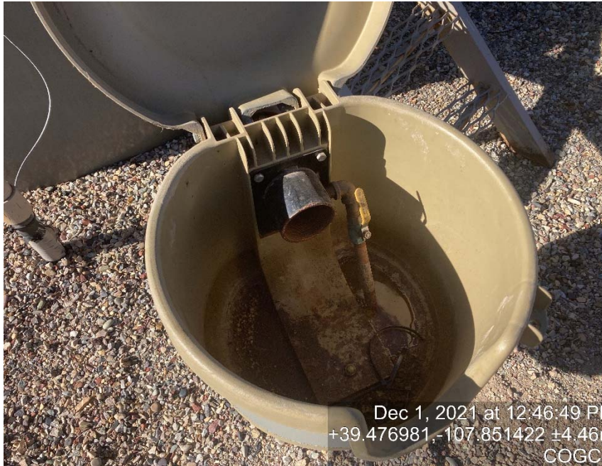
Load out lines missing bull plugs/caps
