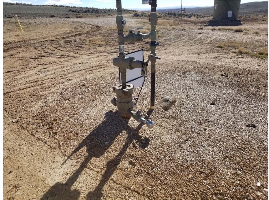
Photo 2. No bradenhead access apparent.
