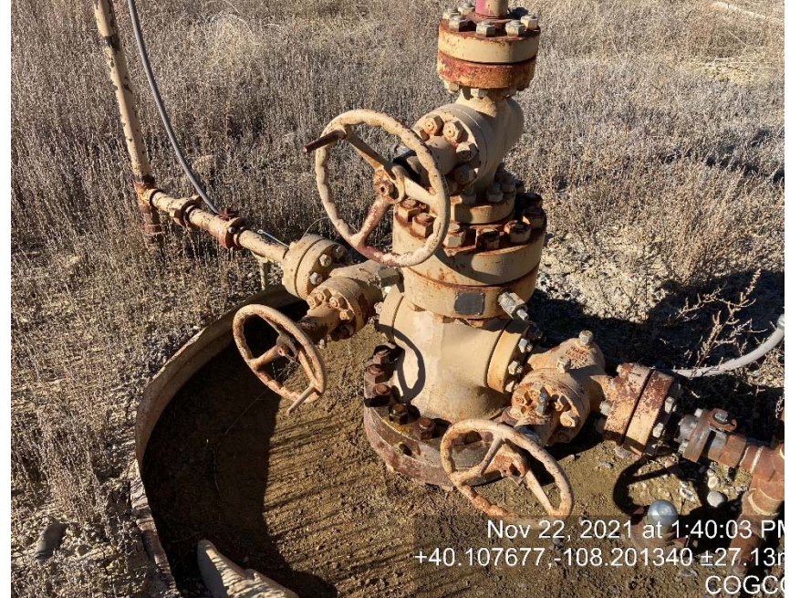
Lack of Braden head access
