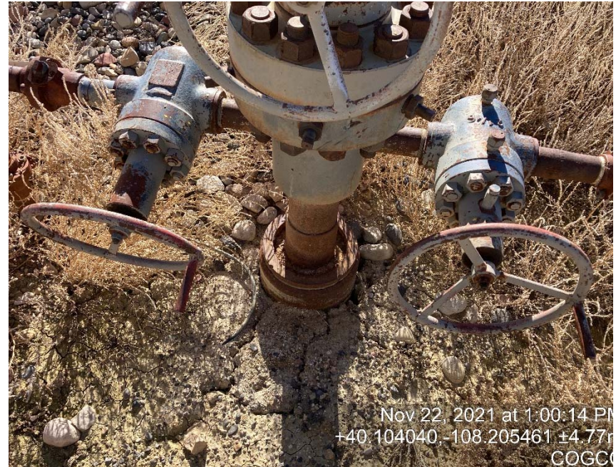
Lack of Braden head access
