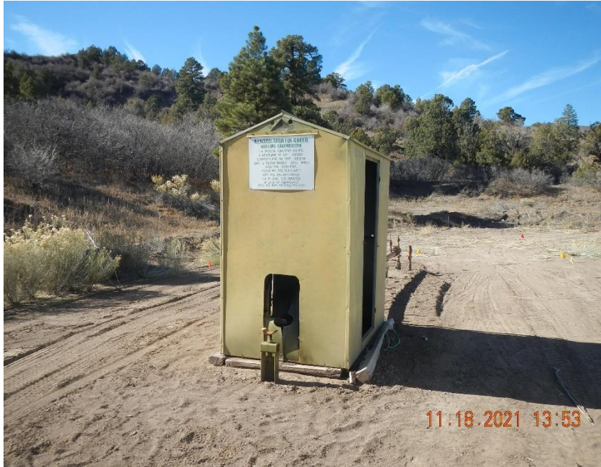
La Posta Canyon #2 meter run. Gathering lines have been disconnected. Flow lines have been marked for removal.
