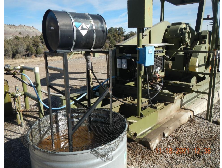
Pump jack skid and surrounding area are wet and stained.
