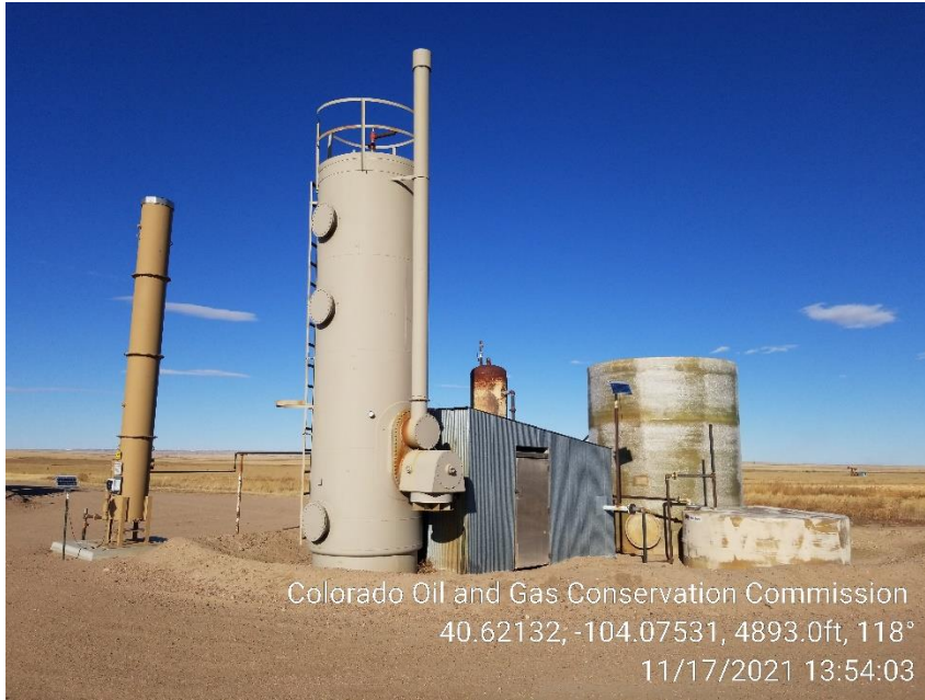
Photo 1 – Heater Treater, ECD, Produced Water Tanks
