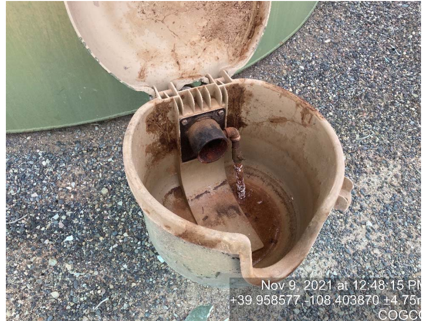
Load out line missing bull plugs/caps
