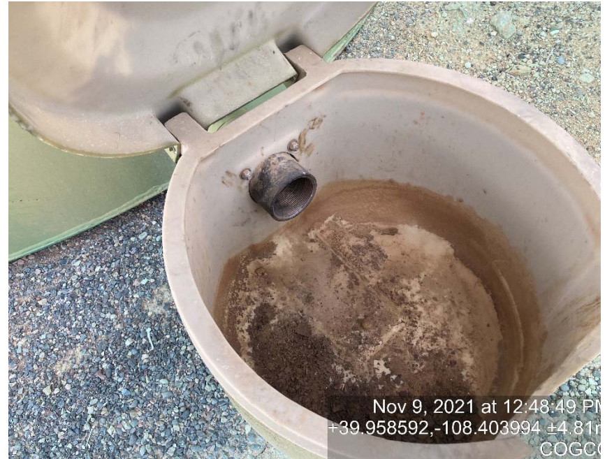
Load out line missing bull plugs/caps
