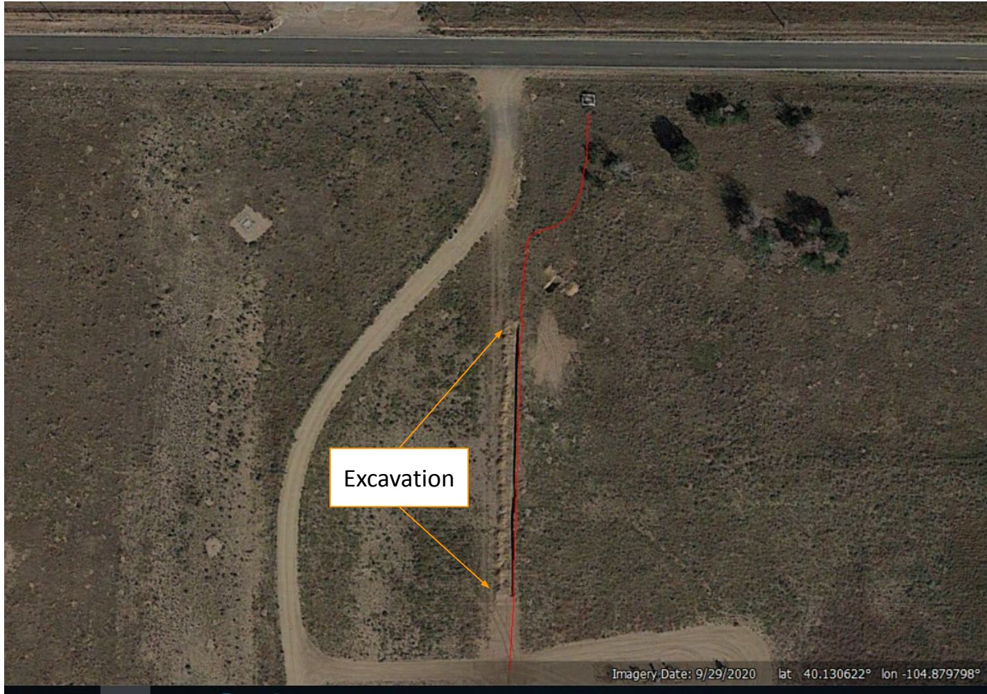
Photo 5. Google Earth aerial imagery taken 9/29/2020. Photo illustrates excavation of what appears to be a flowline. Complainant stated the flowline has subsided. COGCC Staff mapped the subsidence of what appears to be a flowline (red line).
