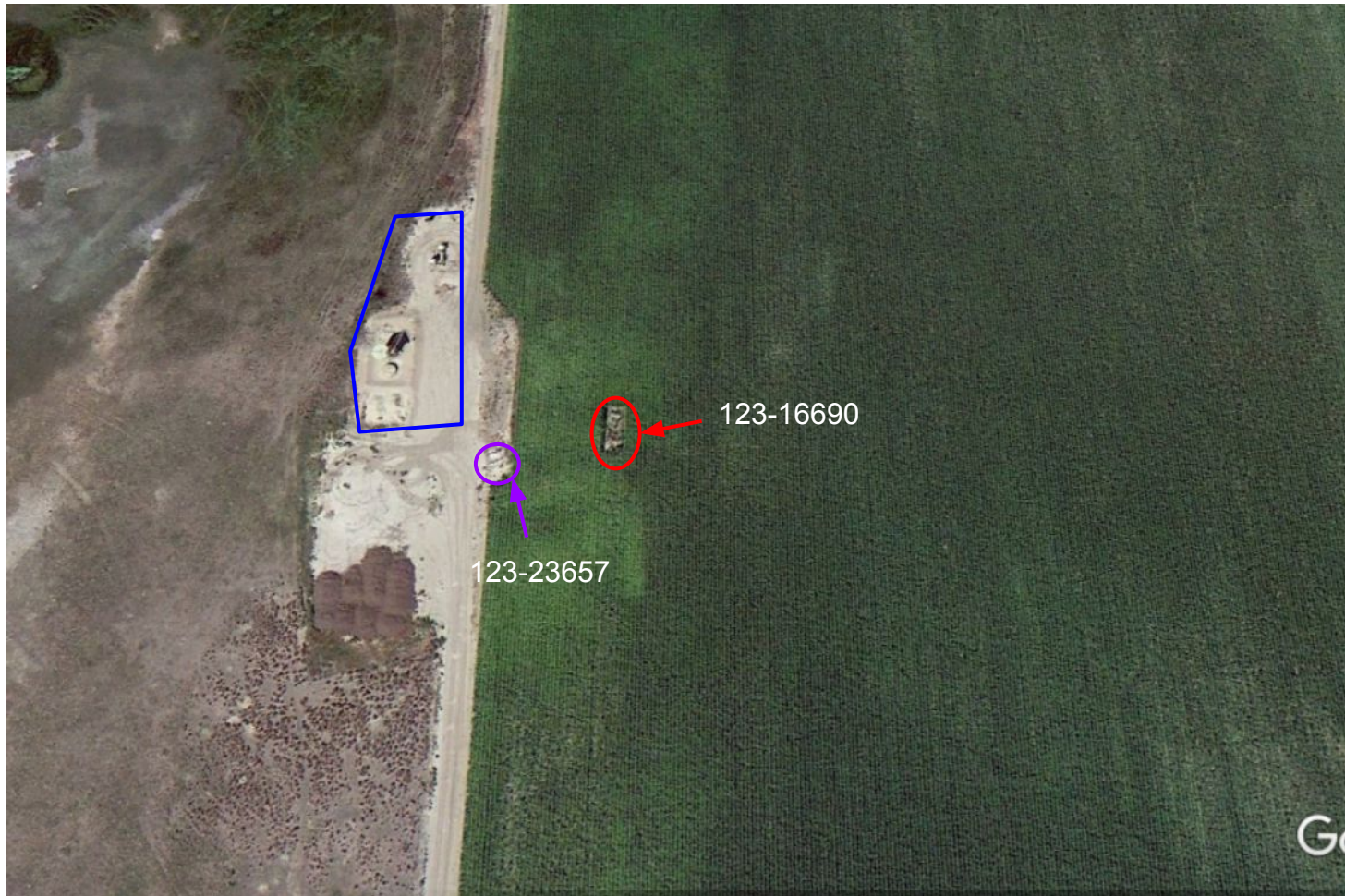
Photo 1. 2012 aerial imagery of the well pad (north is up). The tank battery highlighted in blue will be associated with the temporarily abandoned well API # 123-23657 highlighted in purple.
