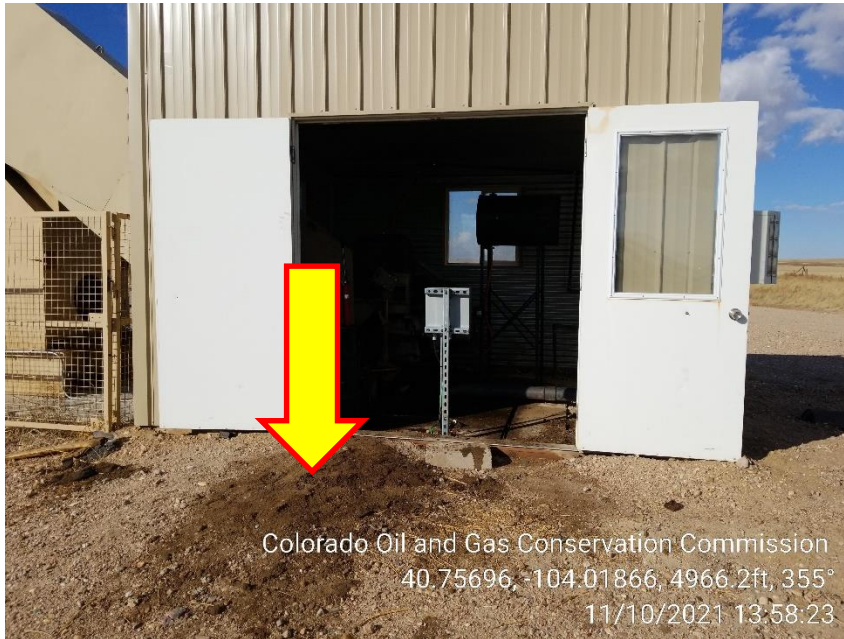
Photo 3 – Stained Soil at Gas Engine
