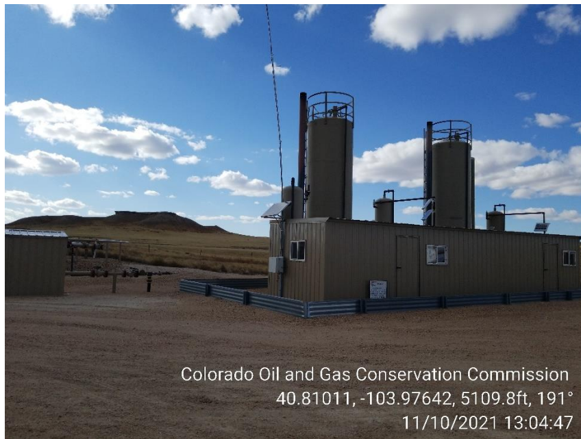
Photo 5 – West Heater Treaters
