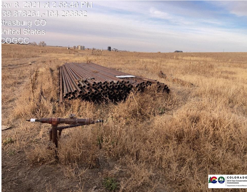
Pic 1 tubing on ground from PA well, risers have not been LOTO
