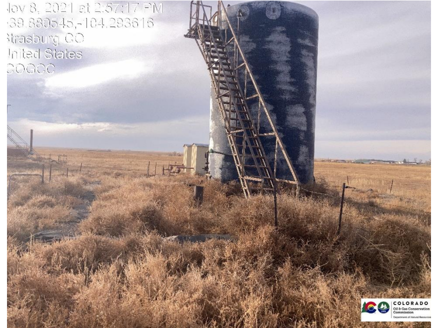
Pic 6 weeds unmanaged, berm needs to be repaired.
