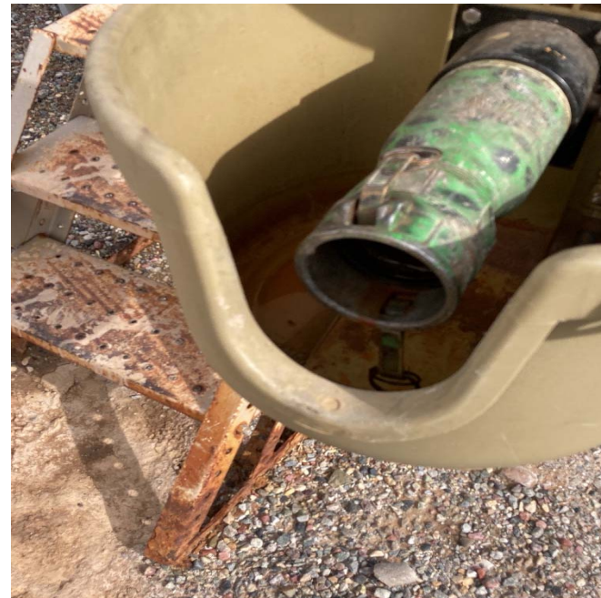
Load line missing cap/bull plug
