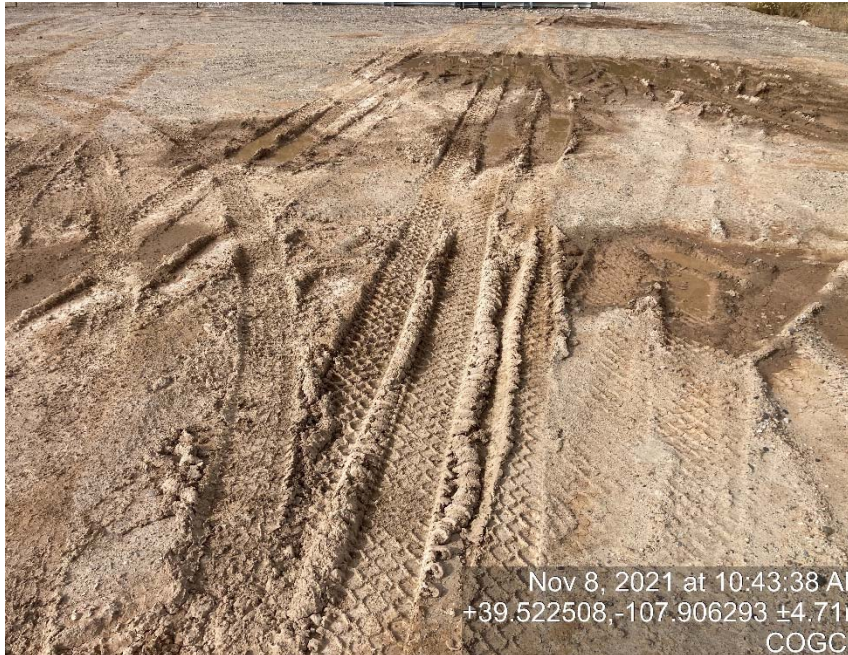
Lack of stabilization/compaction
