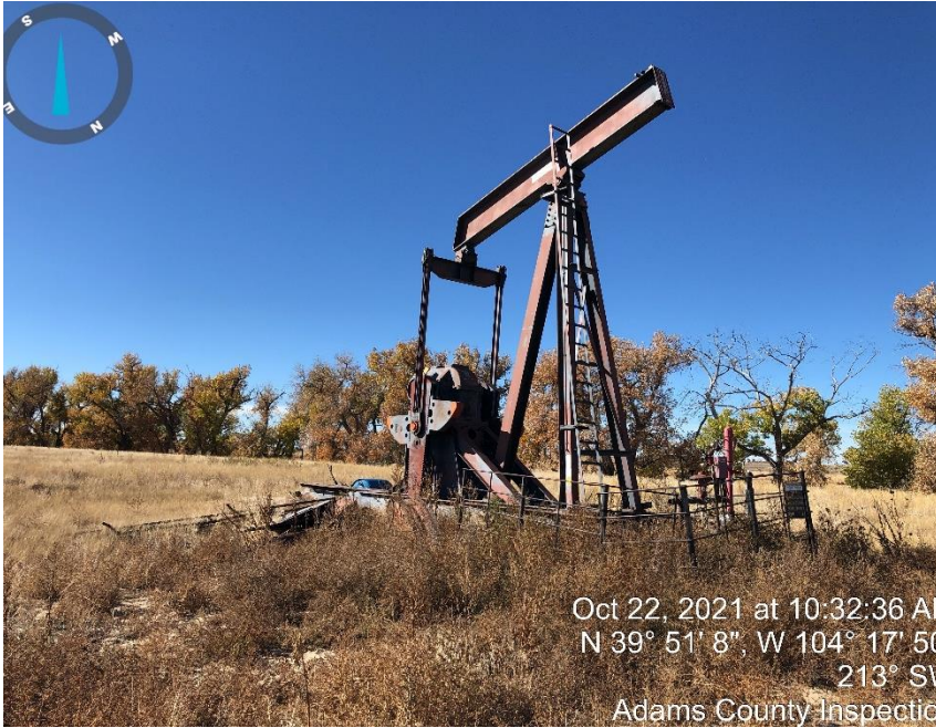
Photo #1 Pump Jack.
