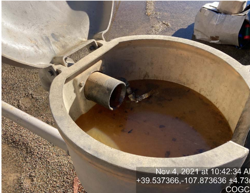
Load out line missing cap/bull plug, leaking and bucket full of fluid
