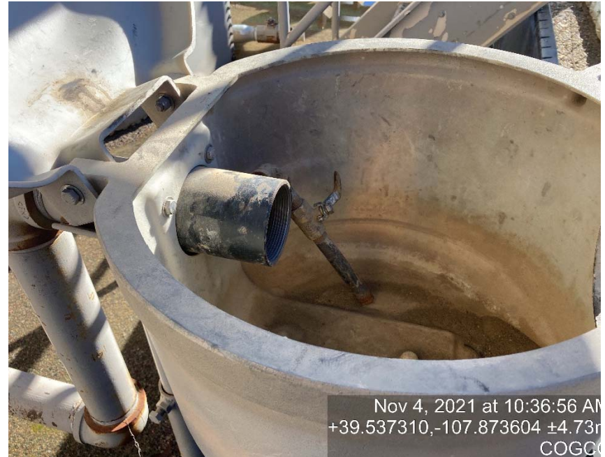
Load out line missing cap/bull plug
