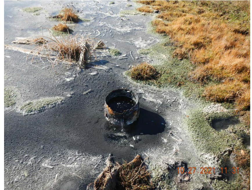
Underwood Ditch (OWP) #5 casing with fluid actively flowing.
