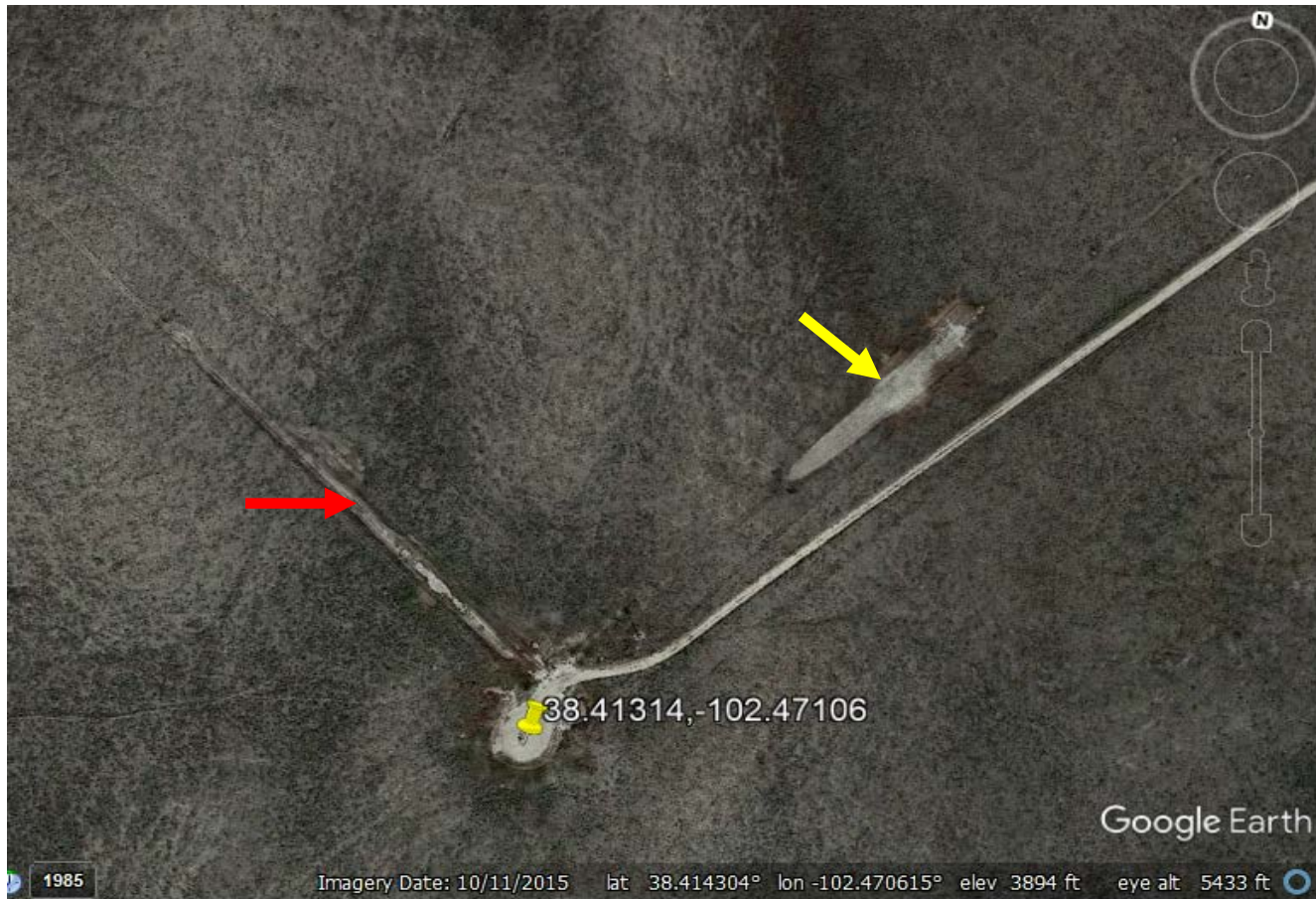
Photo 1. Aerial imagery shows the impacted spill area at yellow arrow and red arrow. There is undesirable weed and bare soil within these area that have not been reclaimed.
