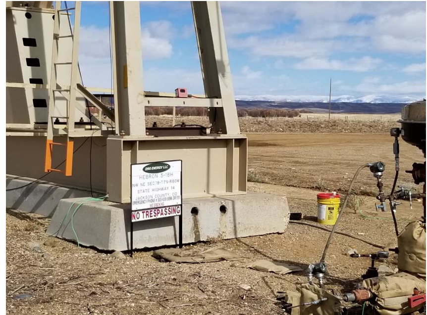
Photo 5. Wellhead sign not updated to current sign rules. Debris on location.
