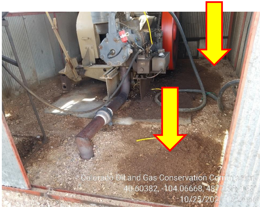
Photo 5 – Stained Soil at Gas Engine
