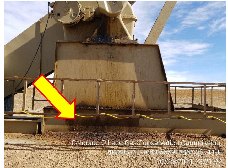
Photo 6 – Stained at Westside of Gearbox
