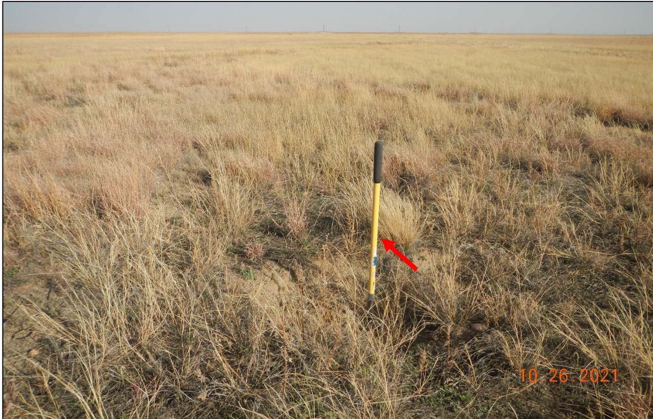
Photo 8. There is an area of subsidence at the location which is approximately 1-2ft. deep. Red arrow points to 5 ft. shovel placed in the area. Approx. Lat/Long:38.85031,-102.39605.
