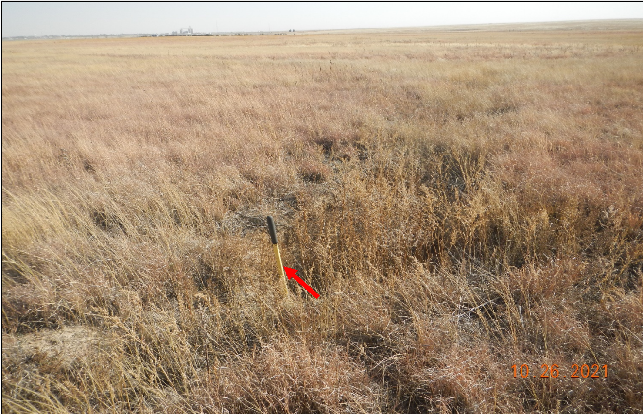
Photo 9. There is another area of subsidence at the north side of the location which is approximately 3-4ft. deep. Red arrow points to 5 ft. shovel placed in the area. Approx. Lat/Long:38.85052,-102.39459.
