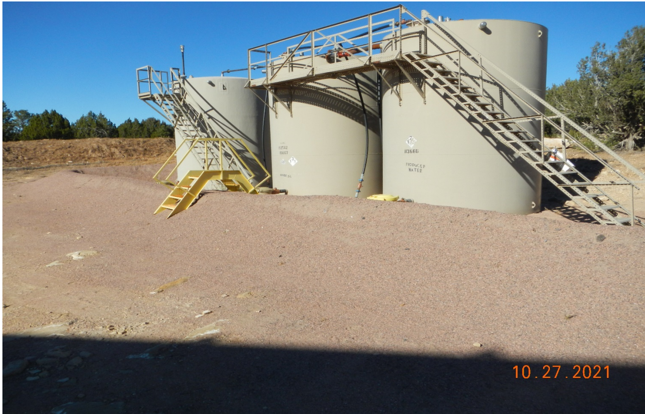
Photo 10. The tanks at north side of the location are not properly labeled.
