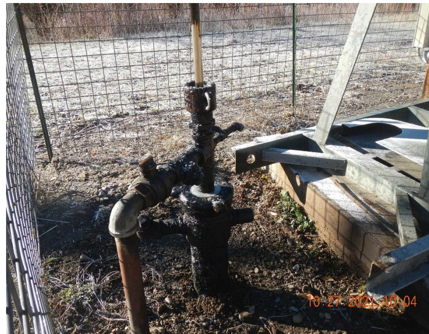
Well head and polished rod are wet and stained with oil.
