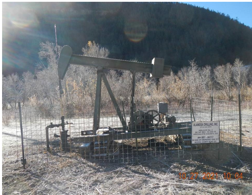
Nielson #4 pump jack and well head. Pump jack was operating during this inspection.
