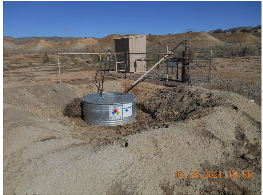
Produced water tank
