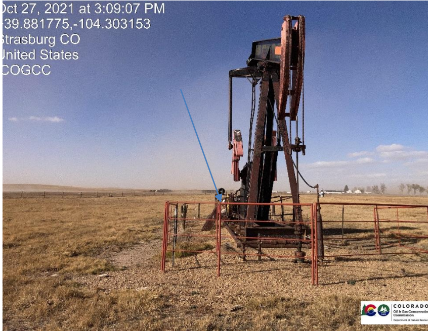
Pic 1 pump jack, guard needs to be attached to pumping unit
