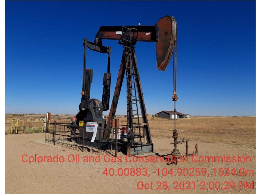
Photo 2 Well head sign falling of and is faded not legible
