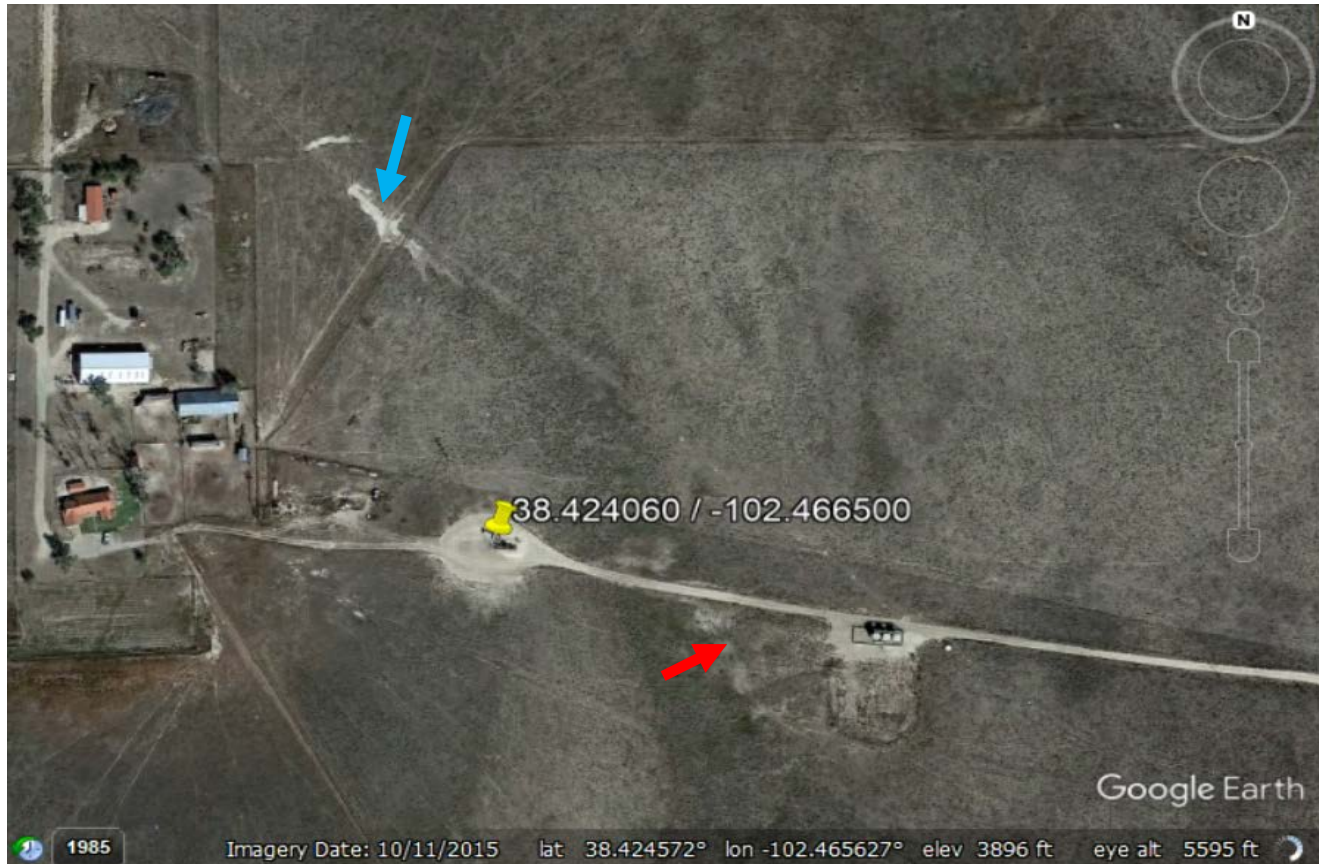
Photo 1. Aerial imagery of the well site and tank battery site. A spill had occurred downhill from the tank battery site shown at red arrow and in the following photos. It appears there was also a spill at the blue arrow north of the well site which was not inspected.
