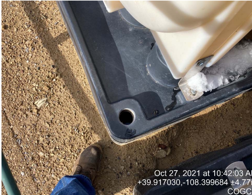
Chemical tank containment is full of fluid
