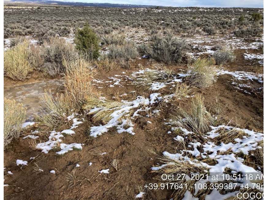
Lack of stabilization/erosion/BMP's failing
