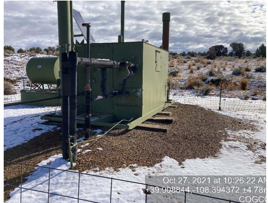
location/Lack of glycol vessel labeling
