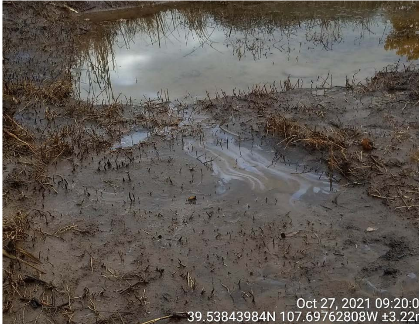
Photo #9 – Localized hydrocarbon sheen observed on surface water located southeast of point of release.
