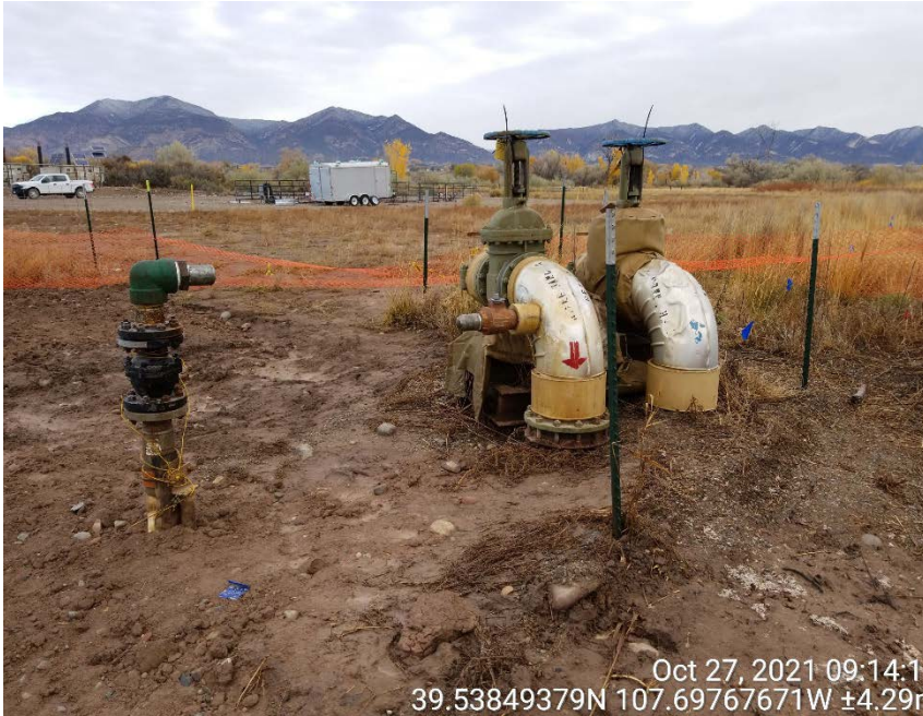
Photo #7 – Flowline risers at the reported point of release for Spill/Release ID #480927.
