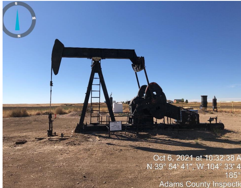
Photo #5 Pump Jack.
