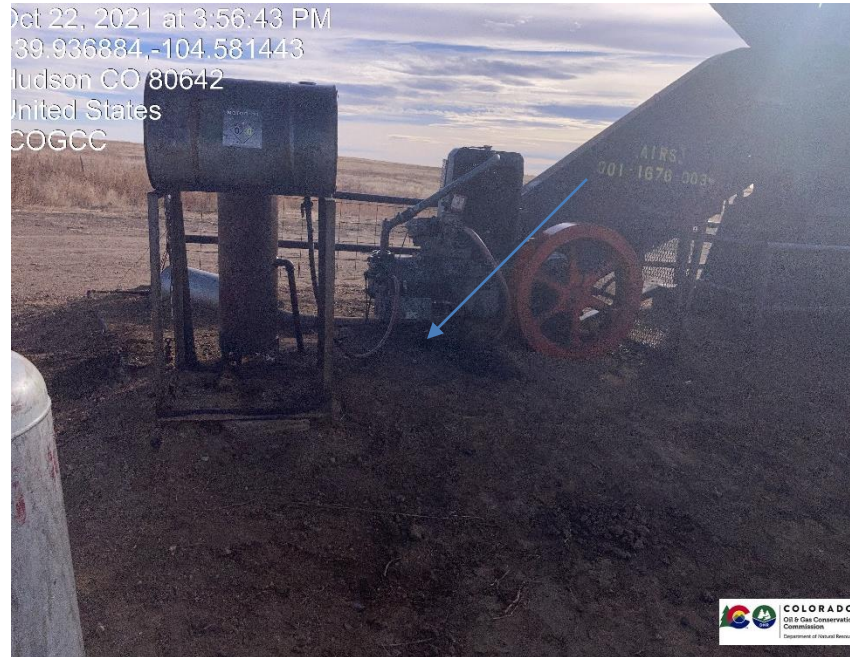
Pic 1 pumping unit motor, stained soil/mechanical issue
