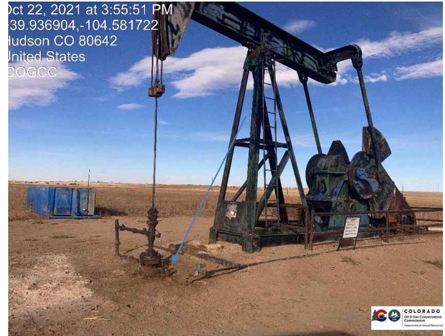
Pic 2 Pumping unit stained soil next to wellhead
