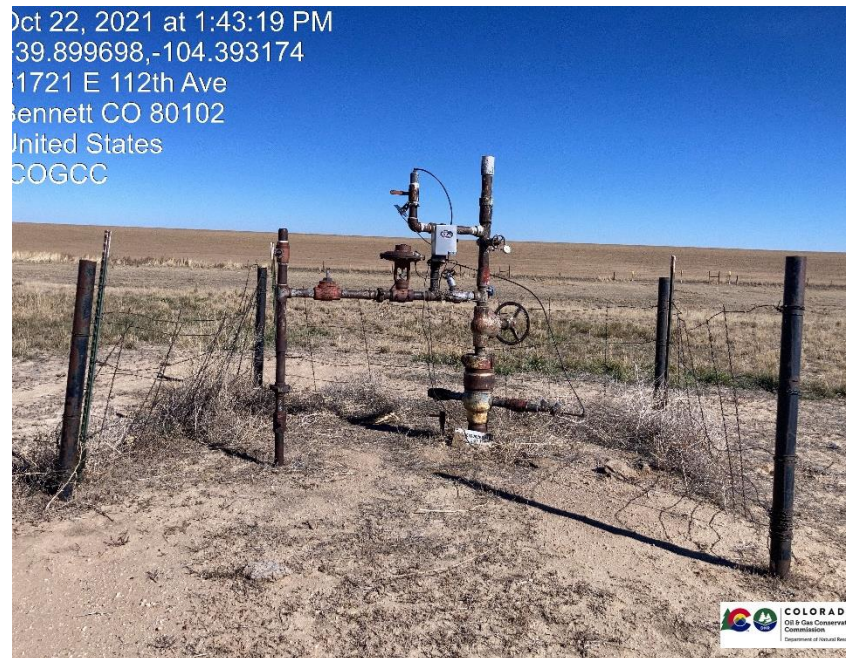
Pic 4 wellhead, weeds unmanaged, sign needs to be placed back on well.
