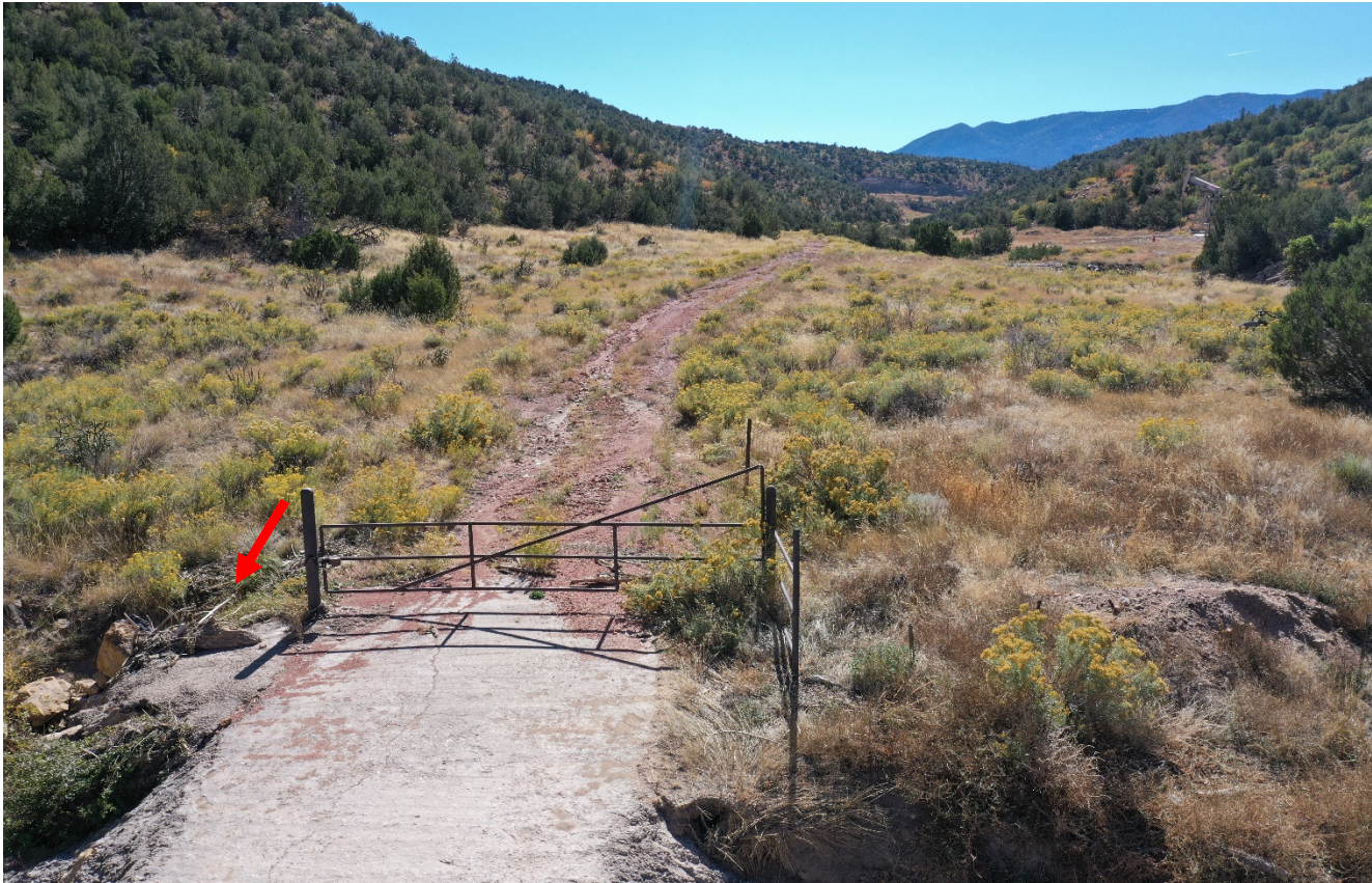
Photo 1. Drone photo facing south toward the access road. There is erosion occurring down the road which is directed toward the stream at red arrow. The erosion along the road has not been repaired or stabilized.
