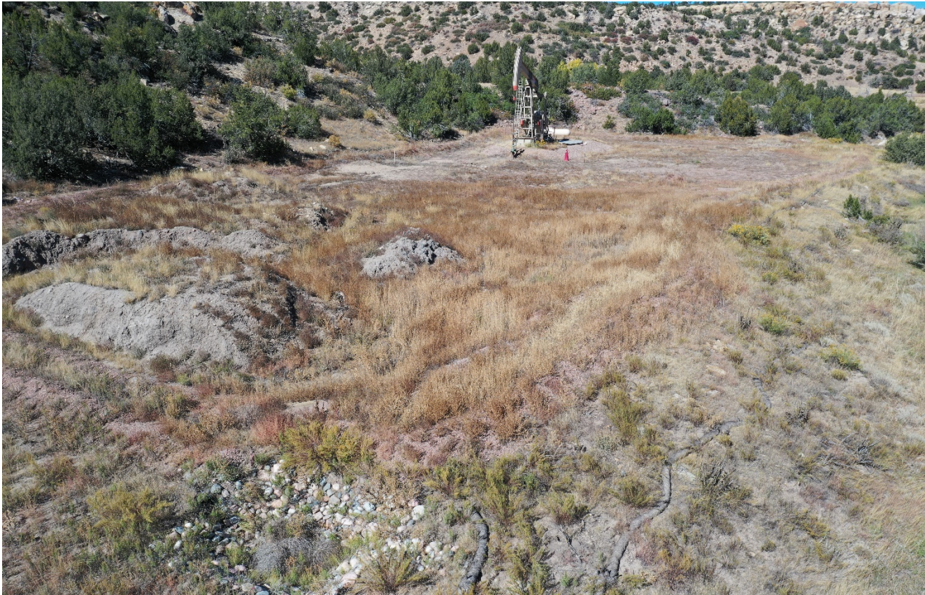
Photo 7. Facing northwest toward the location. Interim reclamation has not been performed. There are undesirable weeds throughout the location. BMP's to control erosion are not maintained.
