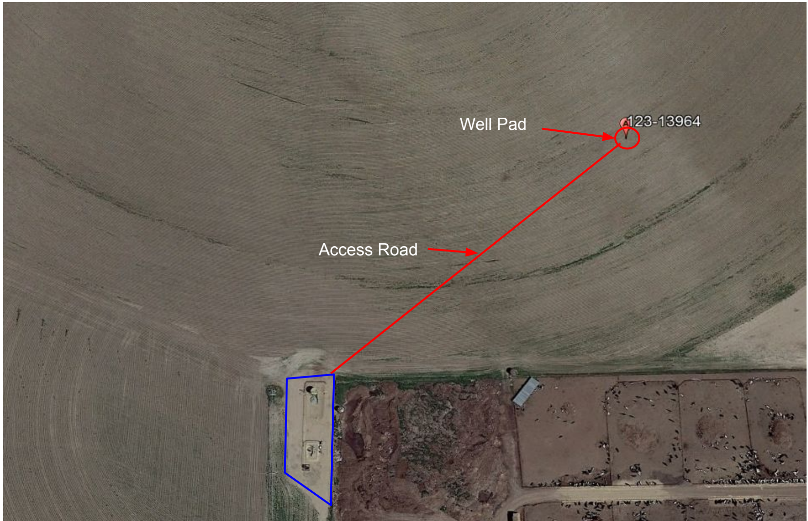
Photo 1. 2021 aerial imagery of the well pad and access road (north is up). The tank battery (highlighted in blue) remains and will be associated with shut in well API # 123-20241.
