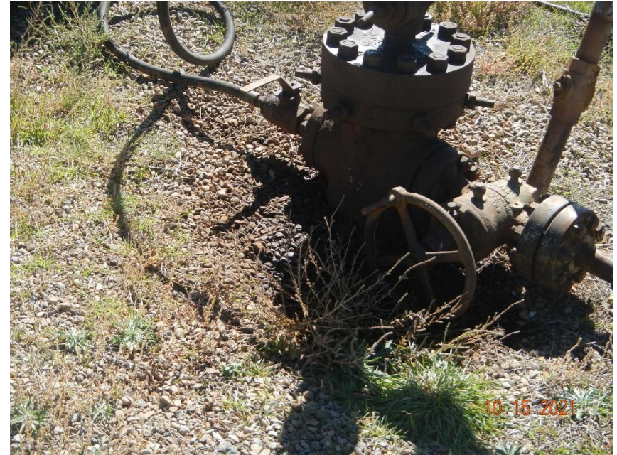
Bradenehead plumbed to surface
