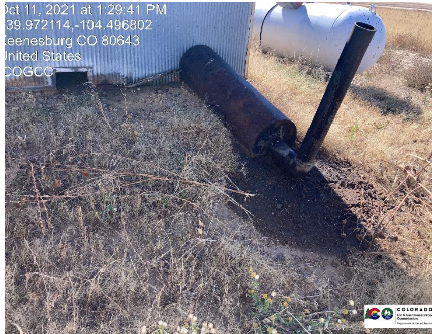
Pic 3 stained soil by pumping unit exhaust
