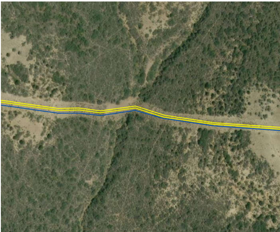
Image 2: Enlarged sections of right-of-way (ROW), showing the location of the water line and the re-vegetation along the ROW. While not fully re-vegetated, there are many sections that are fairly well established in the re-vegetation process. Much of the work would be done on the ROW, not on existing roads, so surficial impact due to removal would be extensive. It also passes under some unmapped drainages.
