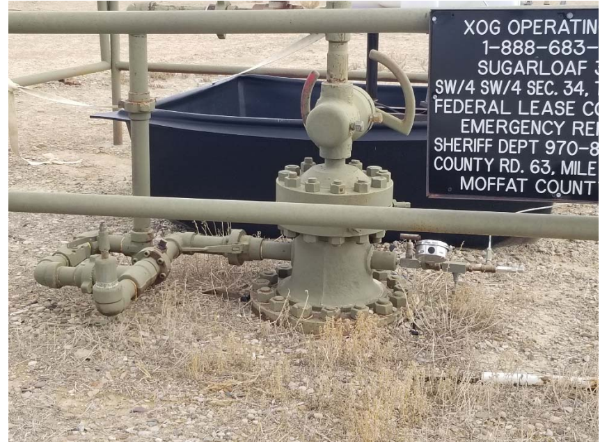
Photo 2. No bradenhead access apparent.
