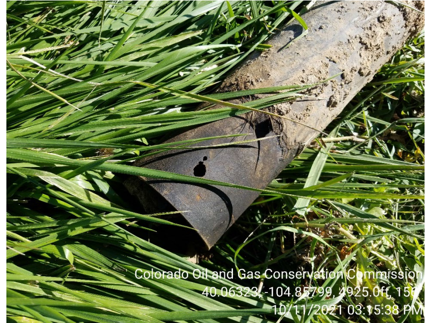
Photo 6 – Hole observed in removed portion of flowline.
