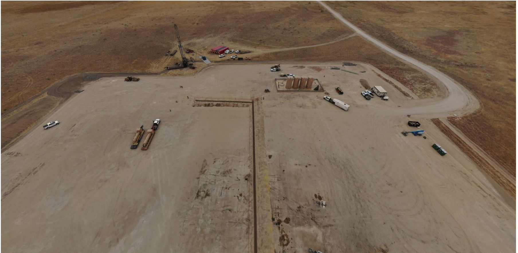
Photo 3. Drone aerial imagery taken from location, facing East. Photo illustrates construction of facilities, plugging operations at an adjacent Tindall well, and the southeast sediment trap.
