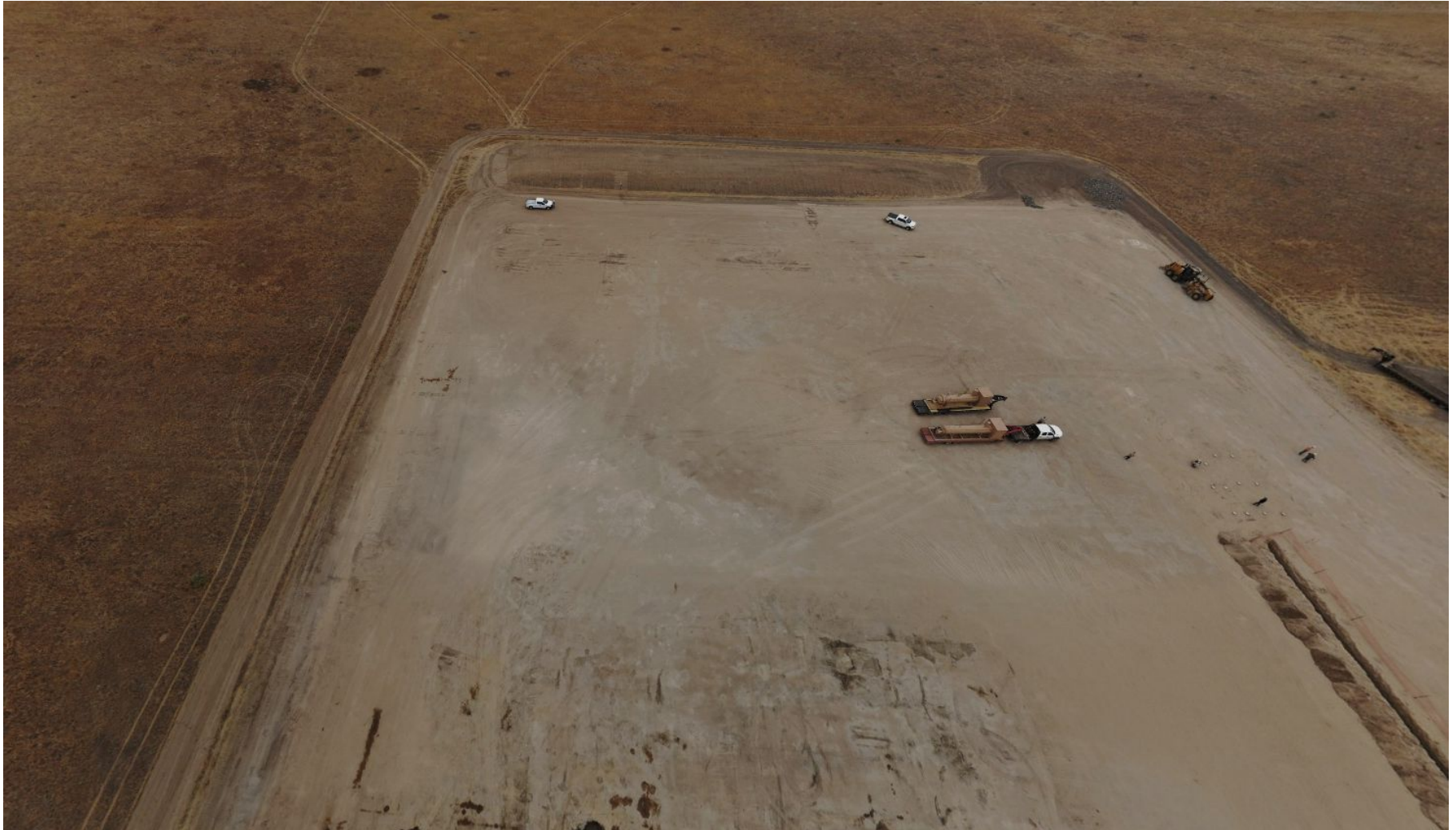
Photo 2. Drone aerial imagery taken from location, facing North. Photo illustrates the topsoil stockpile and northeast sediment trap.
