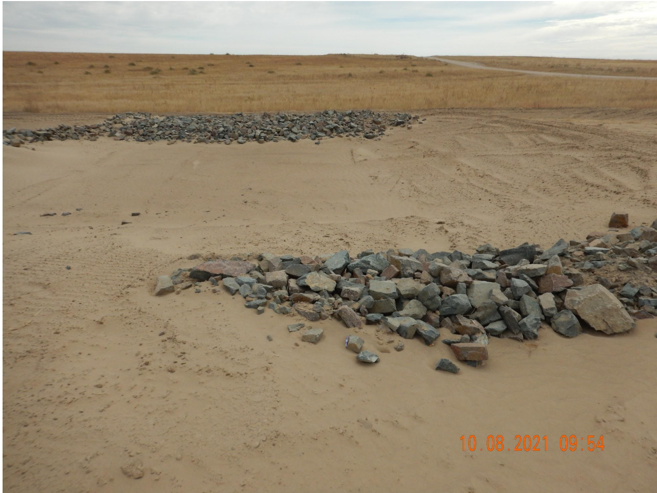
Photo 14. Photo taken of the southwest sediment trap, facing East. Photo illustrates sediment accumulation from unconsolidated soil material from the well location due to wind erosion. The well location has not been properly stabilized.
