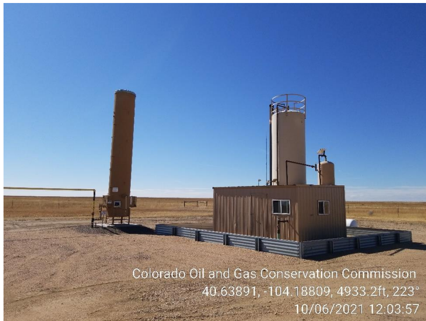
Photo 7 – West Heater Treater and ECD
