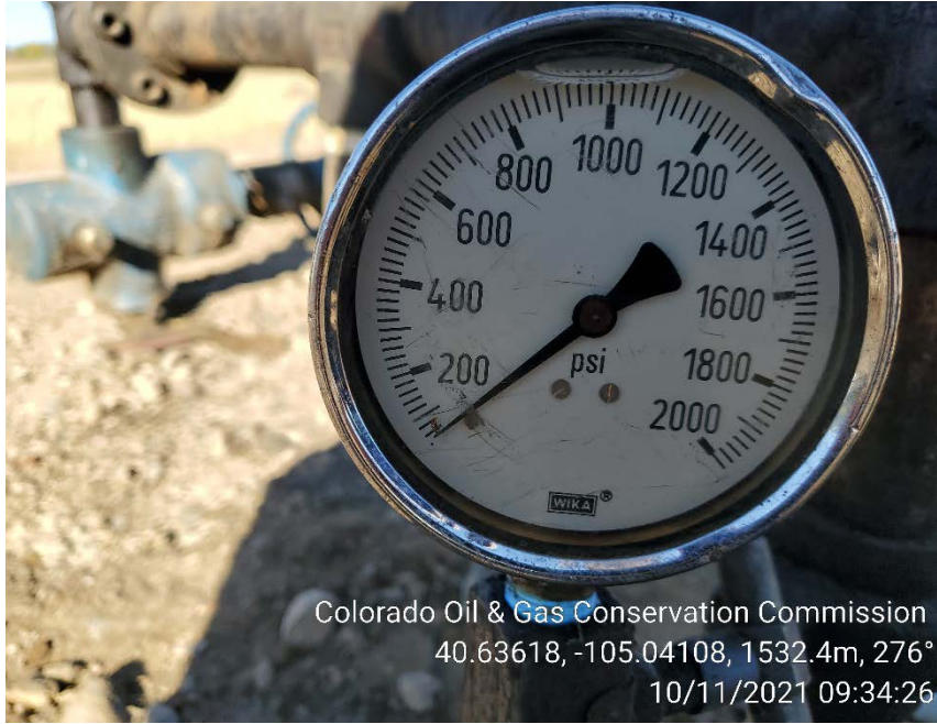
Initial casing pressure
