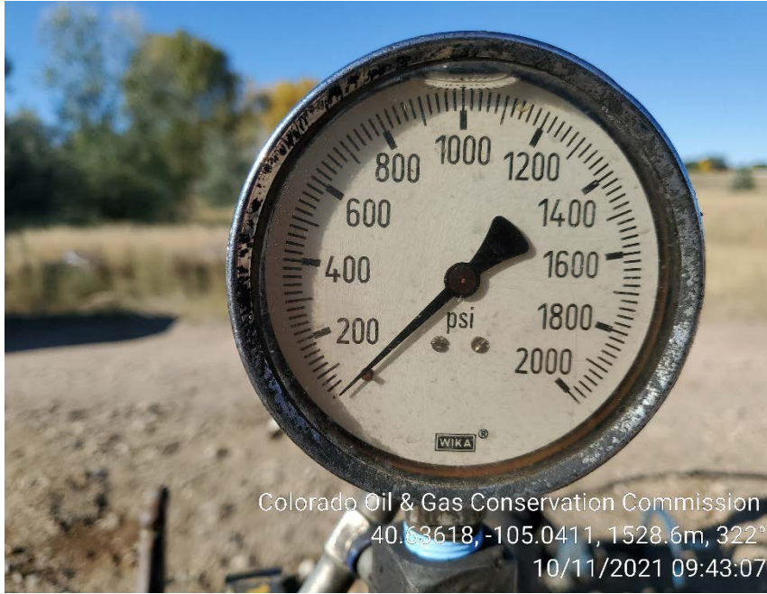
5 minute tubing pressure
