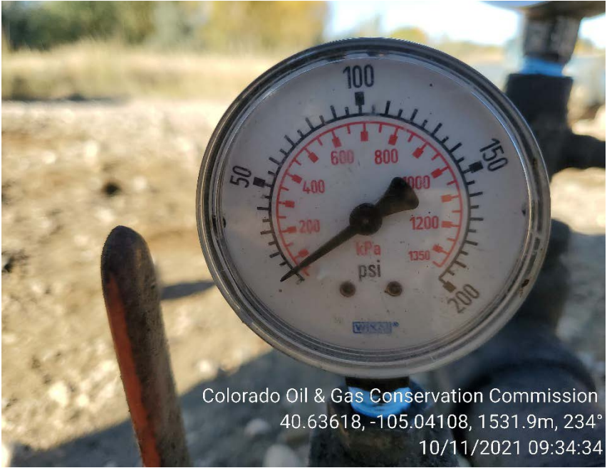
Initial Bradenhead pressure
