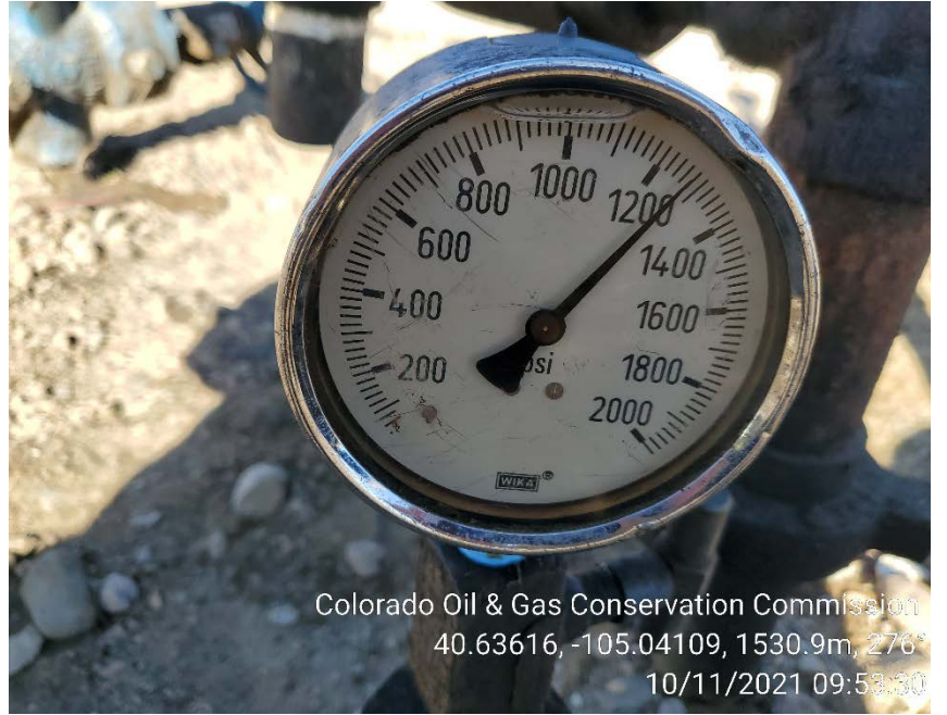
15 minute casing pressure
