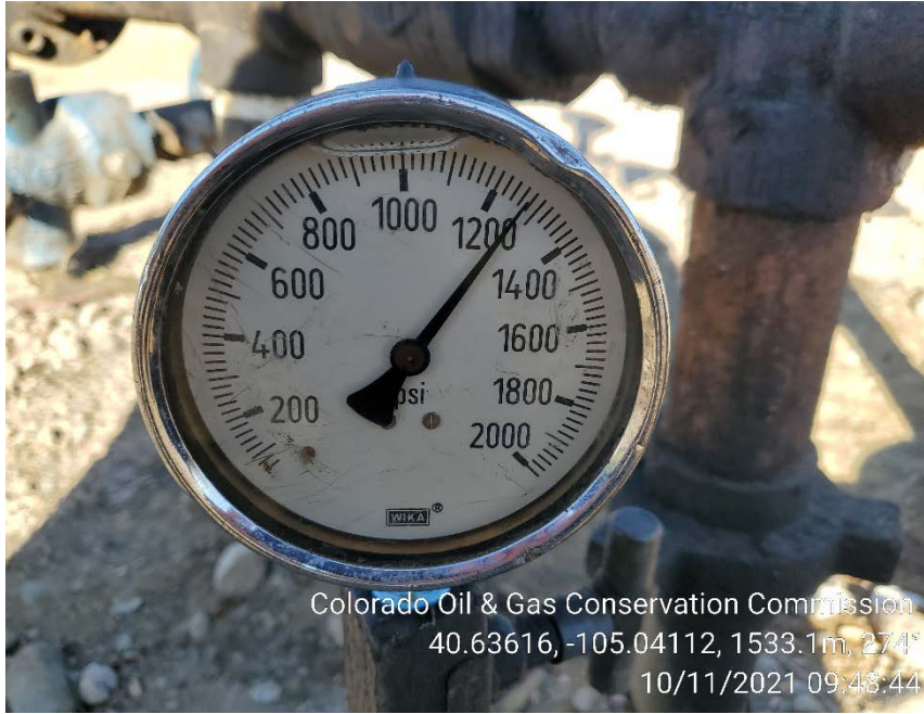
10 minute casing pressure
