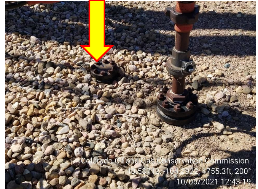
Photo 4 – Unmarked Riser
