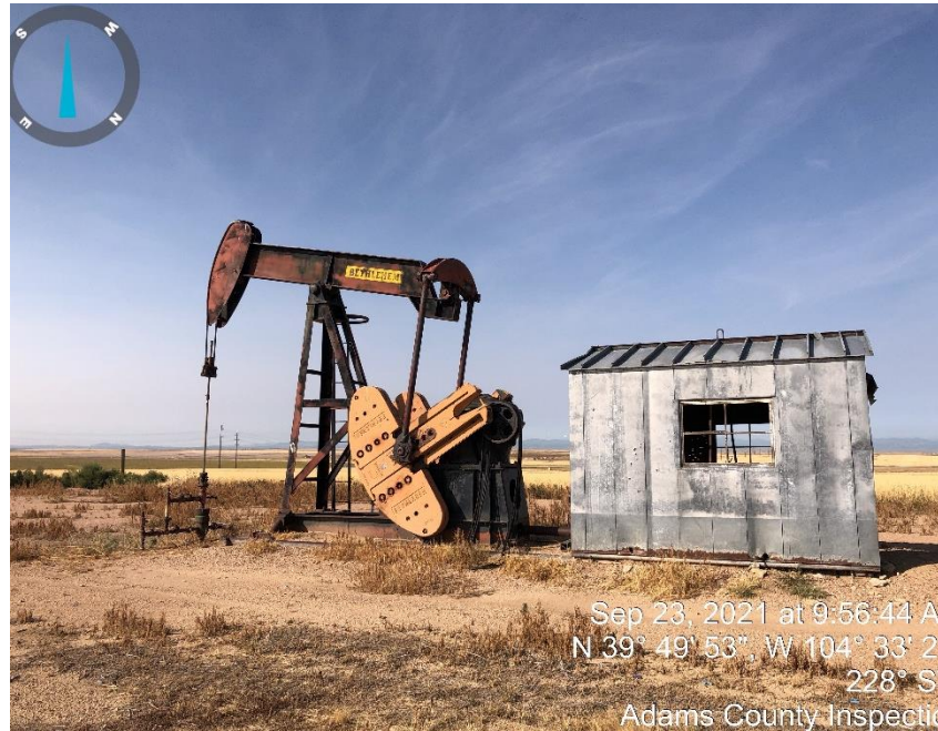
Photo #1 Pump Jack.
