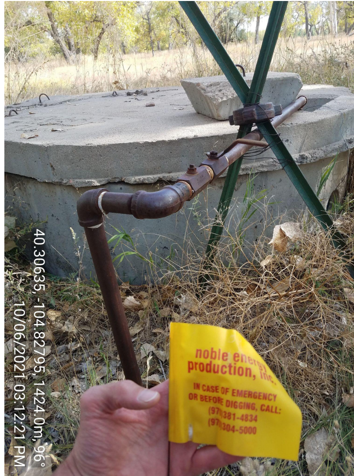
Photo 3. Photo taken from the vault. Photo illustrates Noble locates for flowlines that have not been removed, which includes a vault.
