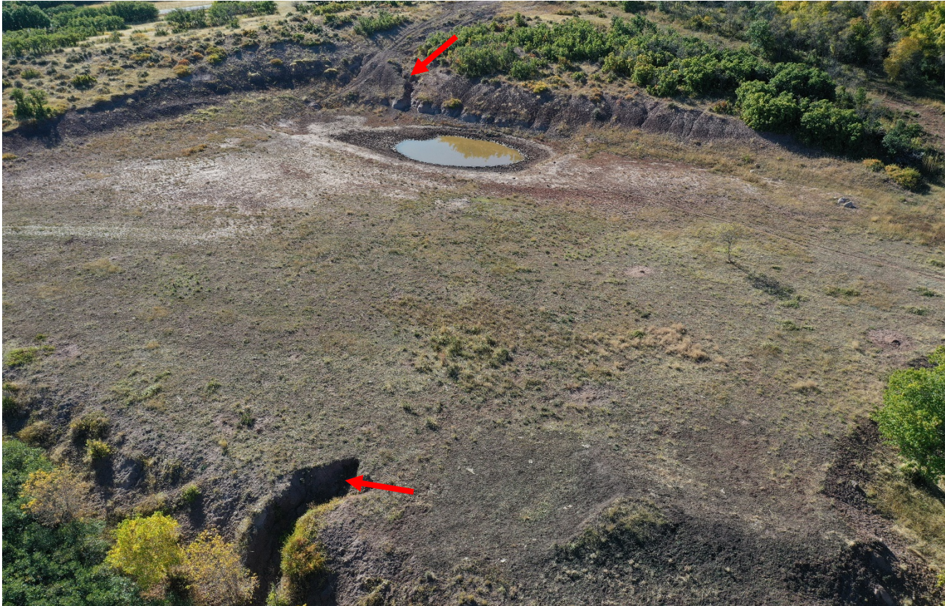
Photo 5. Facing southwest overlooking the location. There are multiple areas of erosion along the cut slope and fill slope shown at red arrows.
