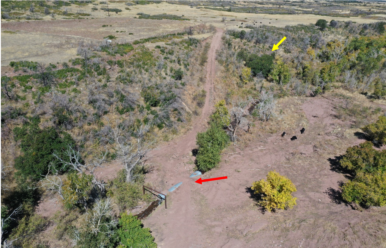
Photo 2. Drone aerial photo facing northeast toward the access road which crossing the perennial stream. The culvert has become exposed due to erosion and is susceptible to further erosion.
