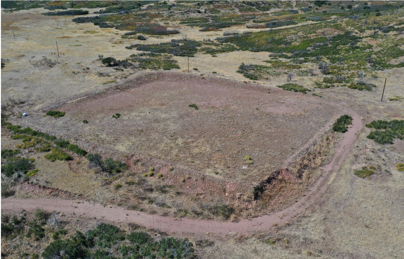
Photo 4. Facing northwest overlooking the location disturbance which is approximately 2.3 acres in size. Aerial image of the location shows the location has not been recontoured and reclaimed.
